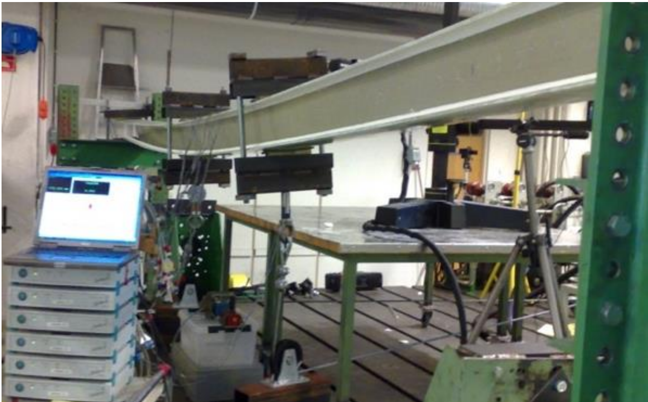
Figure 7 Photo: Bending test of a section on a wing profile. Own photo, from testing
